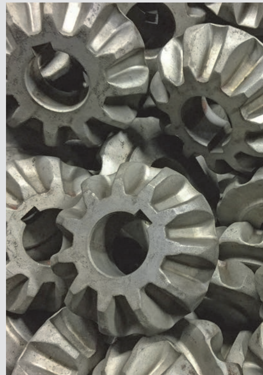
High-strength moulded and tempered gears
