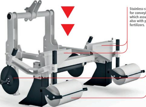
Stainless-steel wide ducts for conveying the fertilizer, which assure high flows also with pelleted fertilizers.
